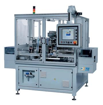
designed for easy use and provides the insertion force and a variety of production data to be collected at an open interface. With a maximum insertion rate of 4.5 cycles per second we provide a production capacity which is difficult to match in the market place. The programmable insertion of two 0.63 mm pins per cycle doubles the output.
