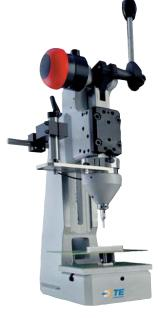
A loose-piece pin or tab is placed in the product specific insertion finger of the arbor press, the PCB is placed on the support anvil and the pin or tab is manually pressed into the board.
