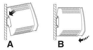
Figure 3 Mounting on a DIN rail
