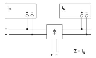
Figure 11 Redundant circuit with redundancy module
