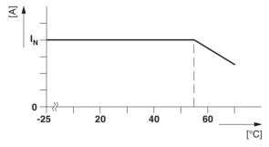
Figure 10 Temperature-dependent derating
