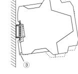
Figure 3 Using the T-BUS DIN rail connector
