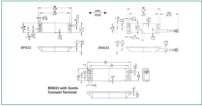
Note: BNS33 reed switch assemblies should be mounted at least 50mm (2") apart.
