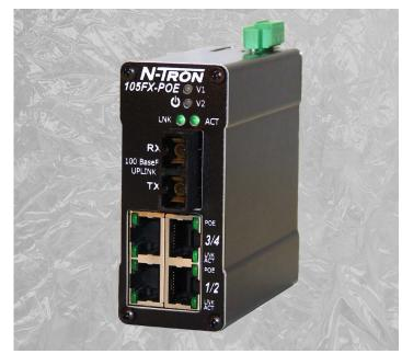
The 105FX-POE auto-negotiates the speed and flow control capabilities of the four TX port connections, and configures itself automatically.
