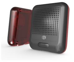
The EL-WiFi-Alert is a standalone monitoring system for all sensor devices in the EasyLog WiFi range. The EL-WiFi-Alert will receive alarm messages from any EL-WiFi sensor device connected to the same wireless network. The EL-WiFi-Alert indicates an alarm activation using high brightness LEDs and a choice of nine alarm tones. The EL-WiFi-Alert continues to work when the PC is turned off.
