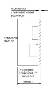
MECHANICAL OUTLINE DIMENSIONS ALL DIMENSIONS ARE IN INCHES [MM] GEN. TOLERANCE: +/-0.02 [+/-0.5]
