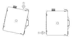
Figure 1 - Attach Data Station To DIN Rail
