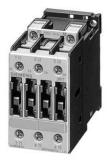
CONTACTOR, AC-3 7,5 KW/400 V, AC 110V 50HZ/120V 60HZ, 3-POLE, SIZE S0, SCREW CONNECTION
