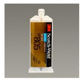
3M<sup>™</sup> Scotch-Weld<sup>™</sup> Acrylic Adhesive DP805 is a two-part MMAbased adhesive. 1:1 mix ratio, 3 minute work life and handling strength in approximately 10 minutes. 3M<sup>™</sup> Scotch-Weld<sup>™</sup> EPX<sup>™</sup> Plus II Applicator and mix nozzles are required (not included).
