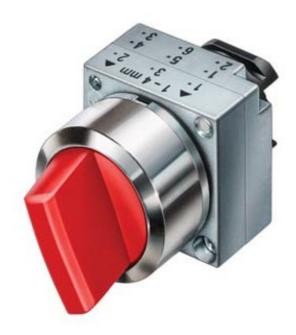
22MM METAL ROUND ACTUATOR: SELECTOR SWITCH LATCHING 3 SWITCH POSITIONS I-O-II NON-ILLUMINATED WITH HOLDER BLACK SOLVENT-RESISTANT
