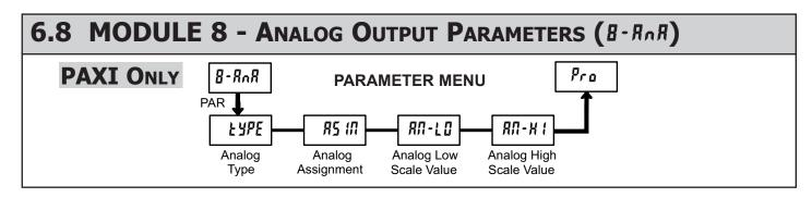
Module 8 is the programming for the analog output parameters. To have an analog output signal, an analog output plug-in card needs to be installed (See Ordering Information). For analog output hardware and wiring details, refer to the bulletin shipped with the plug-in card.
