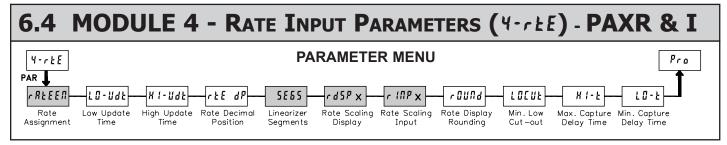
Module 4 is the programming for the Rate parameters. For maximum input frequency, Rate assignment should be set to  $\Pi \mathbf{0}$  when not in use. When set to  $\Pi \mathbf{0}$ , the remaining related parameters are not accessible. The Rate value is shown with an annunciator of 'r' in the Display Mode.
