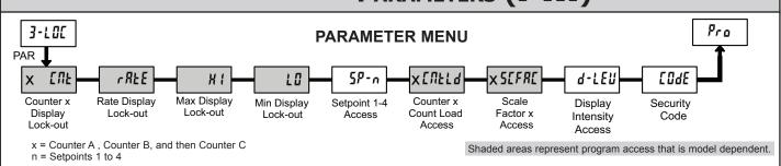
Module 3 is the programming for Display lock-out and "Full" and "Quick" Program lock-out.
