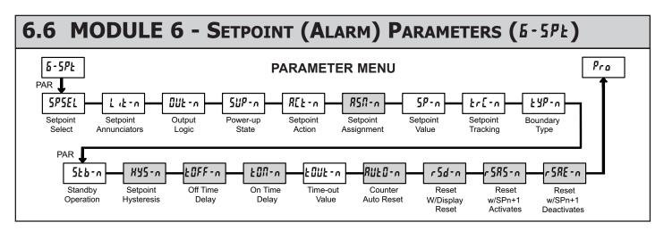
Module 6 is the programming for the setpoint (alarms) output parameters. To have setpoint outputs, a setpoint Plug-in card needs to be installed into the PAX (see Ordering Information). Depending on the card installed, there will be two or four setpoint outputs available. For setpoint hardware and wiring details, refer to the bulletin shipped with the plug-in card. For maximum input frequency, unused Setpoints should be configured for **UFF** action.
