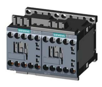
REV. COMB., AC3, 5.5KW/ 400V DC24V 3-POLE, SZ S00 SCREW TERMINAL ELECTR. AND MECH. INTERLOCK
