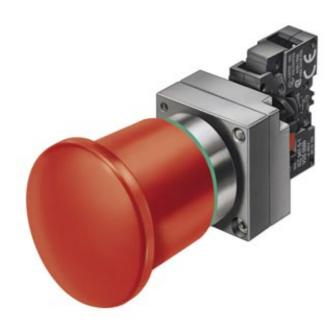
22MM METAL ROUND COMPLETE UNIT COMBINATION: EMERGEN.-STOP MUSHR.PUSHB. 40MM LATCHING W.PULL-TO-UNLOCK MECH. WITH YELLOW BACKING PLATE SCREW TERMINAL, 1NC WITH HOLDER RED SOLVENT RESISTANT INSCRIPTION: EMERGENCY STOP
