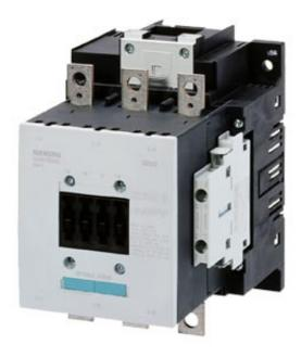
CONTACTOR, 90KW/400V/AC-3, AC(40...60HZ)/DC OPERATION UC 23...26V AUXIL. CONTACTS 2NO+2NC 3-POLE, SIZE S6 BAR CONNECTIONS CONVENT. OPERATING MECHANSIM SCREW TERMINAL
