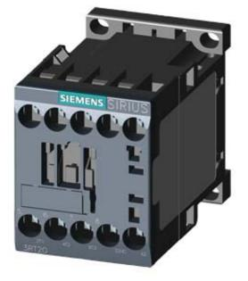
CONTACTOR, AC-3, 5.5KW/400V, 1NC, AC110V 50HZ, 120V 60HZ 3-POLE, SZ S00 SCREW TERMINAL
