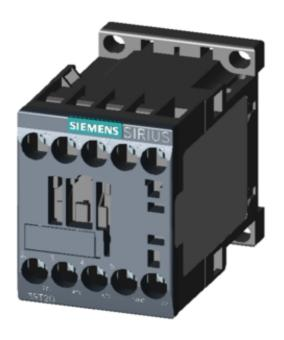
CONTACTOR, AC-3, 5.5KW/400V, 1NO, DC 24V, 3-POLE, SZ S00 SCREW TERMINAL .
