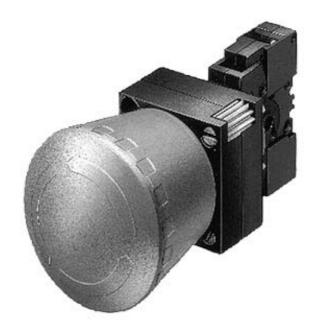
22MM PLASTIC ROUND COMPLETE UNIT COMBINATION: EMERGEN.-STOP MUSHR.PUSHB. 40MM LATCHING W.PULL-TO-UNLOCK MECH. WITH YELLOW BACKING PLATE SCREW TERMINAL, 1NO+1NC WITH HOLDER RED INSCRIPTION: EMERGENCY STOP
