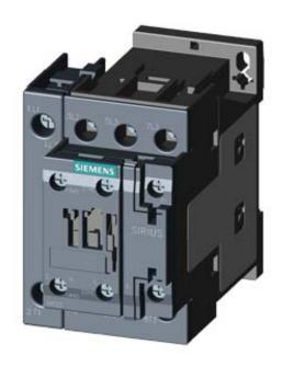
4NO CONTACTOR, AC1: 40A DC 110V 50HZ, 120V 60HZ 4-POLE, 4NO, SZ: S0, SCREW TERMINAL 1NO+1NC INTEGR.
