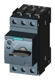
CIRCUIT-BREAKER SZ S00, FOR MOTOR PROTECTION, CLASS 10, A-RELEASE 2.8...4A, N-RELEASE 52A, SCREW CONNECTION, STANDARD SW. CAPACITY
