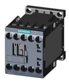
2NO+2NC CONTACTOR, AC3: 5.5KW DC 110V 50HZ, 120V 60HZ 4-POLE, 2NO+2NC, SZ: S00, SCREW TERMINAL
