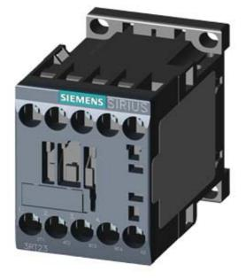
4NO CONTACTOR, AC1: 18A DC 110V 50HZ, 120V 60HZ 4-POLE, 4NO, SZ: S00, SCREW TERMINAL
