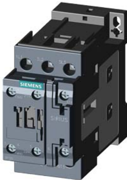
CONTACTOR, AC-3, 15KW/400V, 1NO+1NC, DC 24V, 3-POLE, SZ S0 SCREW TERMINAL
