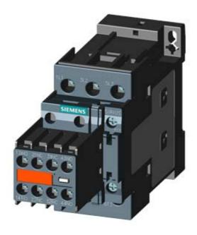
CONTACTOR, AC-3, 7.5KW/400V, 2NO+2NC, DC 24V, 3-POLE, SZ SO SCREW TERMINAL PERMANENT AUX. SWITCH FOR SUVA APPLICATIONS
