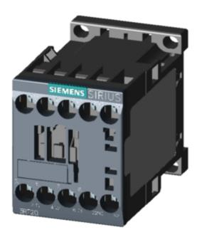
CONTACTOR, AC-3, 5.5KW/400V, 1NC, DC 24V, 3-POLE, SZ S00 SCREW TERMINAL .
