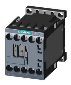
CONTACTOR, AC-3, 5.5KW/400V, 1NO, AC 24V, 50/60 HZ, 3-POLE, SZ S00 SCREW TERMINAL
