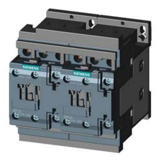
REV. COMB.,AC3, 7.5KW/400V AC220V 50HZ/240V 60HZ 3-POLE, SZ S0 SCREW TERMINAL ELECTR. AND MECH. INTERLOCK 2NO INTEGR.
