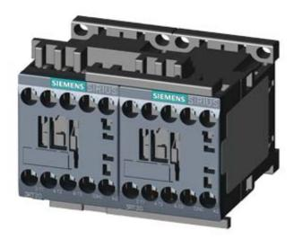
REV. COMB., AC3, 5.5KW/ 400V AC110V 50HZ/120V 60HZ 3-POLE, SZ S00 SCREW TERMINAL ELECTR. AND MECH. INTERLOCK
