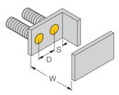
Switching distance not reduced when flush mounted in ferrous metals
