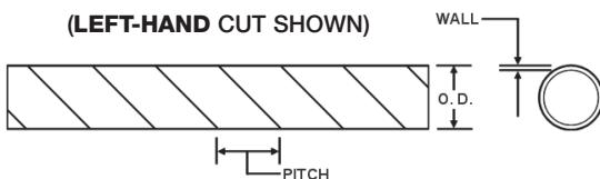
The gripping strength of spiral wrap tubing is enhanced by both its torsional cut and its rigid profile. It retains its strength under repeated flexing and bending and follows wire paths easily, which yields neat, free-running cable bundles. It is extremely useful on long continuous runs where many leads are required; wires can enter or break out at any point. Spiral wrap can be removed easily for troubleshooting and then re-applied.
