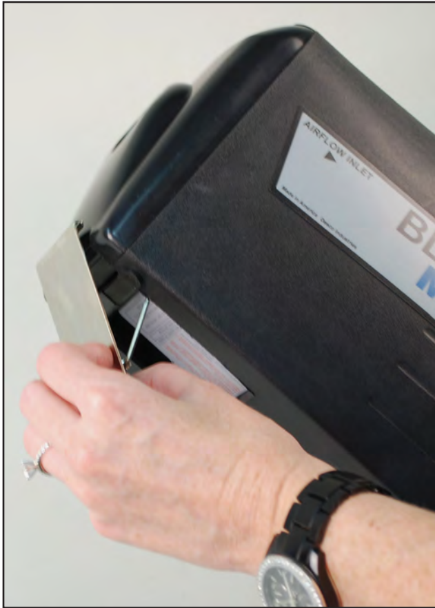
Figure 4: Releasing the Filter
