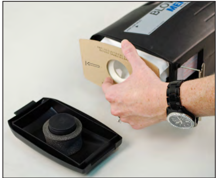
Figure 5: Removing and Changing the Filter
