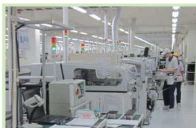
PC board mounting process at NB PTs assembly line of Omron factory
