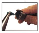
1. Remove wedgelock using needlenose pliers or removal tool. Pull wedgelock straight out.
