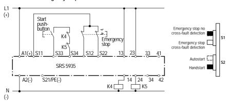
With switching current >10 A, the output contacts should be reinforced by external contactors (K4 and K5) with positive-guided contacts. The proper operation of the external contactors is monitored by looping NC contacts into the restart circuit (terminals S33-S34).
