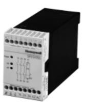
The FF-SRS5935 Emergency Stop modules are designed to be used in emergency stop circuits when danger to personnel or machinery is present. This device has two safety relays with positive-guided contacts to ensure redundancy.
