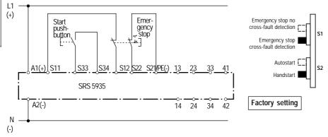
The circuit redundancy in the emergency stop control circuit and therefore gives the highest safety level.
