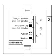
Switches S1 and S2 are used to select **automatic start**, **manual start** and emergency stop with or without **cross fault detection**. These switches are located behind the front cover panel.
