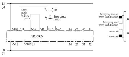
This circuit has no redundancy in the emergency stop circuit.
