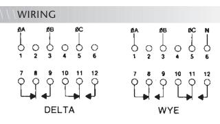
The **PBC Series** offers protection to three-phase equipment that is required to operate between two voltage limits. All three phases are monitored individually for a pre-selected **under** and **over voltage** limit.
