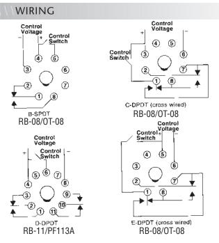
The **Duplexor** is used in control panels where **two loads** are required to alternate to provide equal run time on the loads. The alternating action is initiated by a control switch, which is common with one side of the control voltage. The output contacts will change states each time the control switch is opened, thus alternating the two loads. The LED indicators show the position of the output relay.
