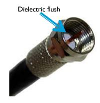
4) Twist until cable is fully seated. When white dielectric is flush with the bottom of the nut connector is fully seated.
