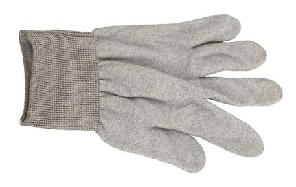
A properly grounded operator can touch a charged ESD sensitive device and a damaging ESD event can occur (Charged Device Model). Increasing the electrical path's contact resistance is one way to control the speed of the discharge and reduce the possibilities of damage. A good way to accomplish this is by wearing static dissipative gloves.
