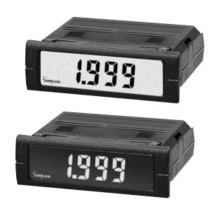
Simpson's Mini-Max Current Indicators provide high quality, accuracy and reliability in a compact, 60mm deep case. Units offer 3-1/2 digit, 0.5" (12.7mm) LCD display and are available with a bright red, negative image backlight option. All units feature user-selectable decimal point, auto zero and limited scaling capabilities.
