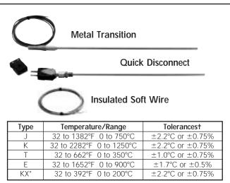
\*Extension Wire-Type For Fahrenheit, multiply tolerance in °C by 1.8.
