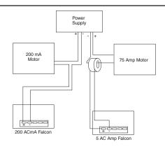
the front bezel. Adjust potentiometer VR101 until the display indicates 75.0 (amps) when the 5 amp signal is on. Replace the bezel, and remove the signal. The transformer is installed on one of the legs of the motor
