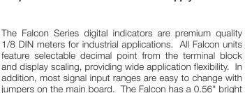
Compactly designed for applications requiring minimal rear panel depth, the Falcon fits a standard 1/8 DIN panel cutout (91.9mm x 45mm) and requires less than 3" behind the panel. A screw terminal connector is a standard feature for easy wiring of the power supply and signal input connections.
