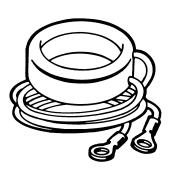
Donut Current Transformers enable the Falcon to monitor AC current up to 1999 amps. The Donut (also known as a "Toroid") is placed around one of the legs of the device being monitored, and emits up to a 5 amp signal. The Falcon can be scaled to accurately display the current being monitored.
