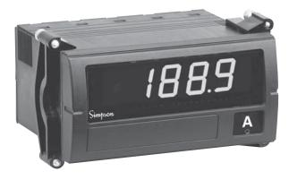
Compactly designed for applications requiring minimal rear panel depth, the Falcon fits a standard 1/8 DIN panel cutout (91.9mm x 45mm) and requires less than 3" behind the panel. A screw terminal connector is a standard feature for easy wiring of the power supply and signal input connections.
