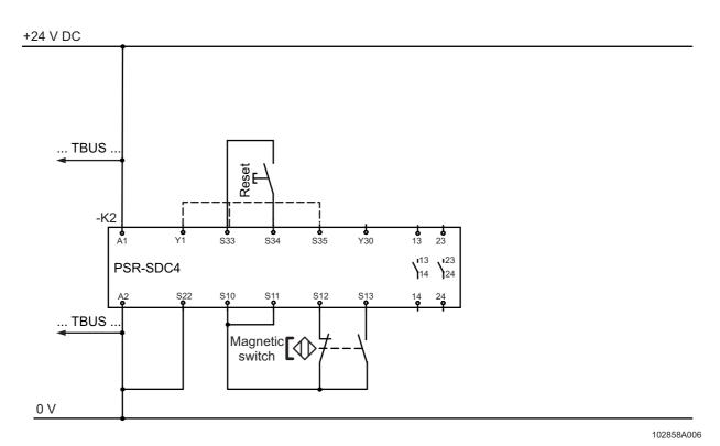
Figure 9 Monitoring with encoded magnetic switch without cross-circuit detection, with closed safety door
