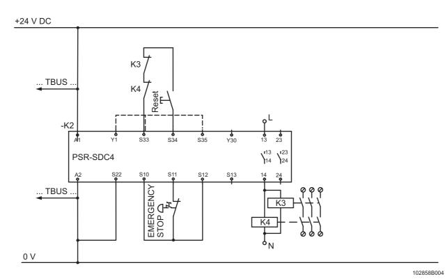
Figure 11 Single-channel emergency stop circuit with monitored contact extension
