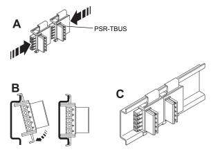
Figure 3 Using the T-BUS DIN rail connector
