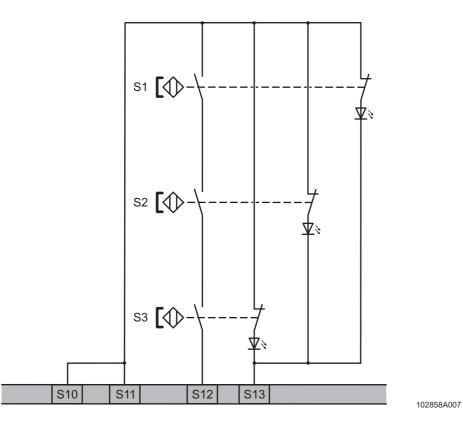
Figure 10 Connection for safety category 3 according to EN 954-1: Example with three magnetic switches with 2-pos. control switch (N/C contact and N/O contact), with open safety door
