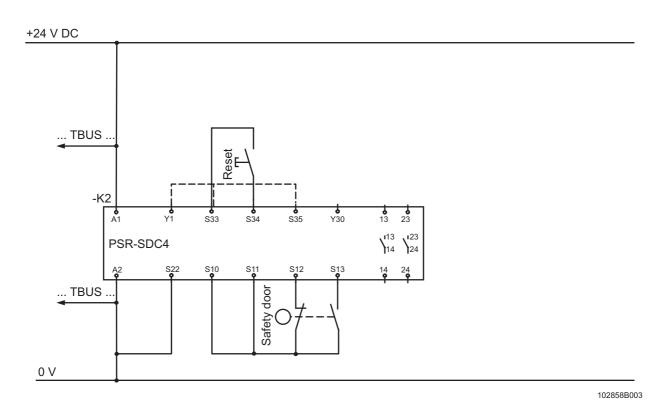
Figure 8 Two-channel safety door monitoring without cross-circuit detection, one N/C contact and one N/O contact
