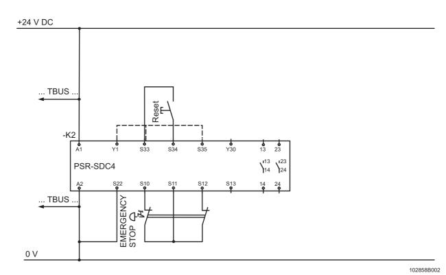
Figure 7 Two-channel emergency stop circuit without cross-circuit detection
