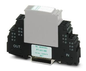
Base element for protective plug PT with protective circuit for 4 signal wires, with gas-filled surge arrester between the connections 3-4 (GND) and 9-10, for mounting on NS 35/7.5 and NS 35/15, housing width: 17.5 mm
