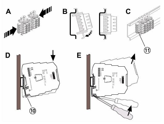
Figure 5 Mounting/Removing
