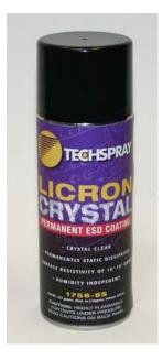
Licron Crystal<sup>™</sup> is a revolutionary and innovative concept in permanent static dissipative coatings. It provides excellent adhesion to metals, glass, plastics, paints and most other surfaces. Licron Crystal operates from 0-100% humidity. The cured coating is durable, will not chip and maintains 10<sup>7</sup>-10<sup>9</sup> ohms resistivity. Licron Crystal is crystal clear, unlike other static dissipative coatings (including the original Licron) that are translucent.
