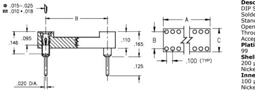
Description: DIP Socket Solder Tail Standard Solder Tail (0.125 Tail) Open Frame Through Hole Accepts .015-.025" Leads Plating Code:
