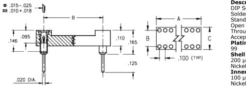
Description: DIP Socket Solder Tail Standard Solder Tail (0.125 Tail) Open Frame Through Hole Accepts .015-.025" Leads Plating Code: oo
