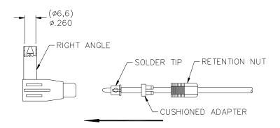
6. ASSEMBLE SOLDER TIP AND CUSHIONED ADAPTER. ALINE THE BANANA PLUG THRU HOLE TO SOLDER TIP. THREAD BY SLIDING SOLDER TIP ASSEMBLY INTO BANANA PLUG THRU HOLE AND TIGHTEN RETENTION NUT TO RIGHT ANGLE.
