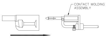
H PUSH FIT ASSEMBLY INTO FRONT MOLDING, CHECK FOR PROPER LATCHING.
